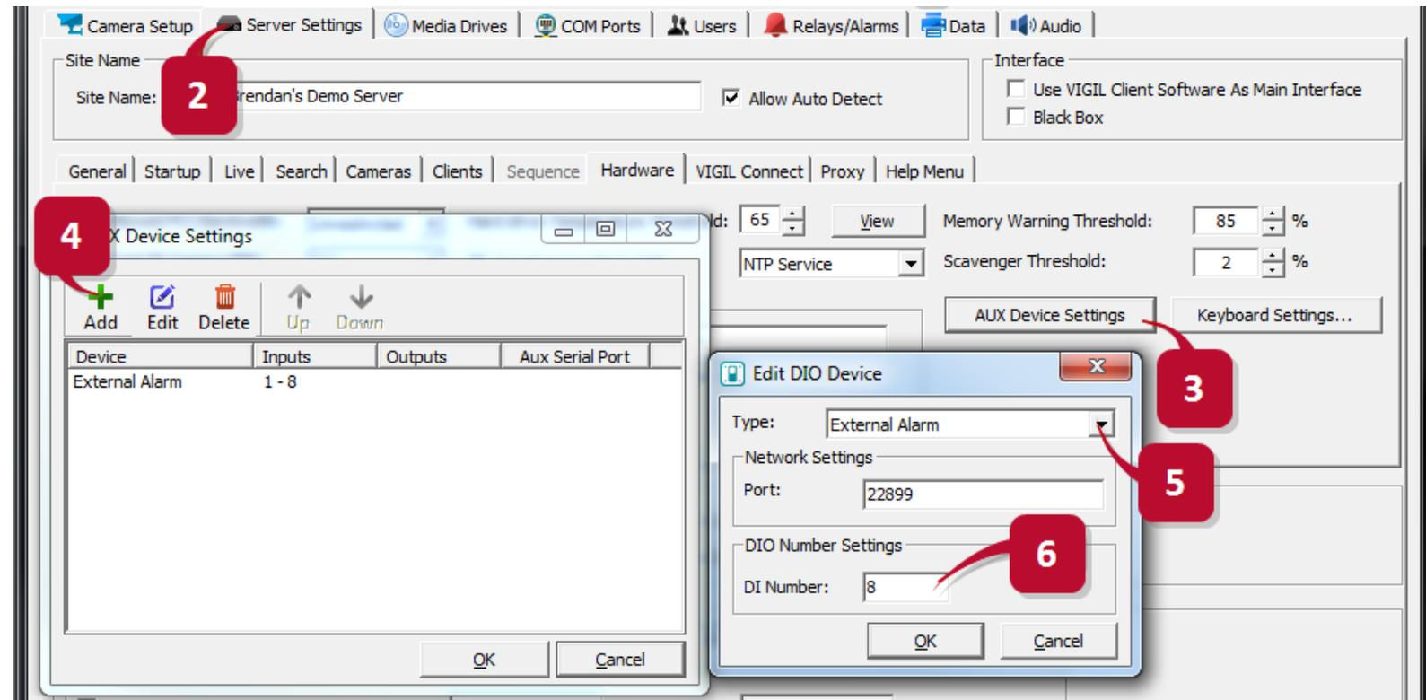
**Figure 8-1:**Configuring VIGIL Relays for use with ANPR Utility- Configuring AUX Settings in VIGIL Server
