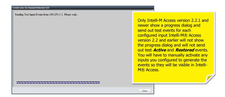
While the progress window is visible, the device will send an *Active* and a *Restored* event for each input you designate. Events are sent *only* for those channels designated as inputs. These events will then be added to the Intelli-M® Access event database, allowing you to act on one or more of these events on the Rules Page.
