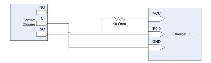
The above diagram will provide a low voltage signal while the contact closure is open, and a high voltage signal when the contact is closed. The reverse behavior can be achieved by moving the wire from the NC connection on the contact closure to the NO connection.
