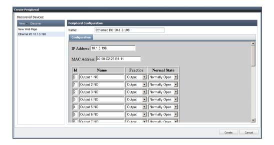
If you selected a device that you created manually, then simply modify the Name field to match what you want Intelli-M® Access to know the device by, and click the *Create* button at the bottom of the dialog. This will finalize the process of creating a Peripheral for the Ethernet I/O device in Intelli-M® Access.
