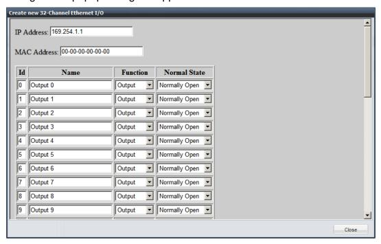
A non-functional default IP Address of 169.254.1.1 will be displayed, along with a default MAC Address of 00:00:00:00:00. Enter the correct IP Address and MAC Address of the device you wish to add.
