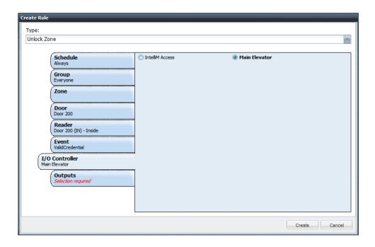
Finally, choose the Zone you wish to be unlocked when Main Elevator's Input 1 activates.
