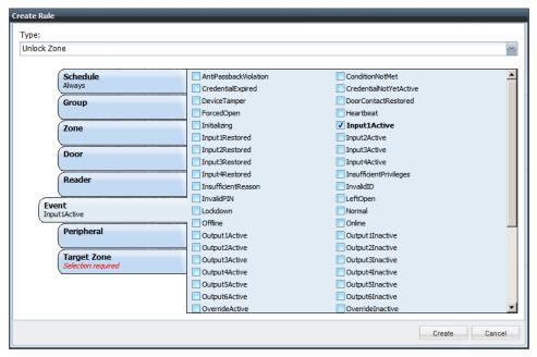
Click on the **Peripheral** Tab and select the **Ethernet I/O** device whose Input 1 you wish to use to activate the Unlock Zone Rule.
