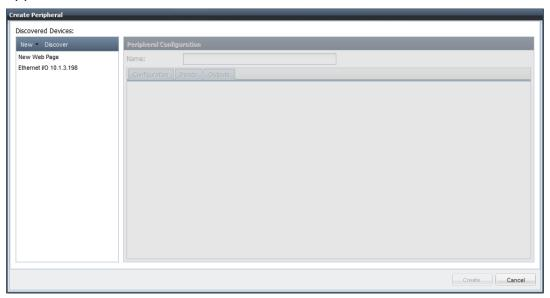
If your Ethernet 32 Channel I/O devices are in the same subnet as the Intelli-M® Access server, they will automatically be discovered, and you will see those device(s) listed on the left pane, as shown in the figure above. The figure above shows a single discovered Ethernet I/O device. If you do not see the device you are looking for, then click the *New* menu and select *32-Channel Ethernet I/O* from the menu.
