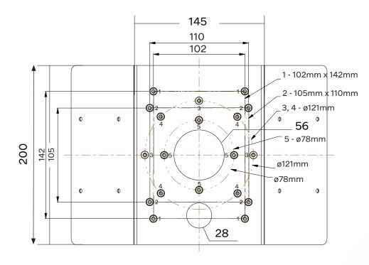
Mount Point 1: 102mm x 142mm Mount Point 2: 105mm x 110mm Mount Point 3-4: Ø121mm Mount Point 5: Ø78mm
