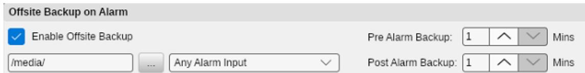
The screenshot shows a form titled 'Offsite Backup on Alarm'. It includes a checked checkbox for 'Enable Offsite Backup'. Below it is a text input field containing '/media/' followed by an ellipsis button. To the right is a dropdown menu with 'Any Alarm Input' selected. Further right are two spinners for 'Pre Alarm Backup' and 'Post Alarm Backup', both set to '1' with 'Mins' to their right.
