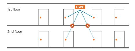
When planning, keep in mind that items can create interference that may reduce range. Items such as: Wi-Fi access points, metal furniture, (shelving and cabinets), HVAC equipment, elevators and microwave ovens all can cause interference.
