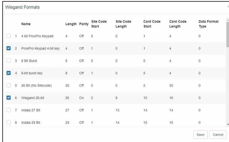
Figure 76: Enable Wiegand Formats
