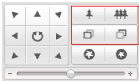
Figure 6-31 Zoom/Focus Adjustment via PTZ Interface
