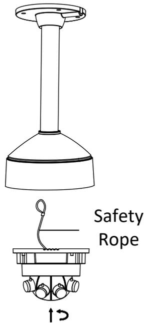
Figure 8-19 Install the Camera to the Bracket (1)
