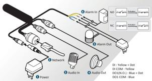
• Power Connection Please check the voltage and current capacity of rated power carefully.
