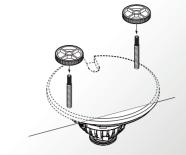
Insert the mount bolts into template holes after connecting the cables. 6 Fix the camera by tightening mount nuts to
