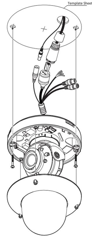
**1** Disassemble the camera. See the "Disassemble the Camera" section for more info.
