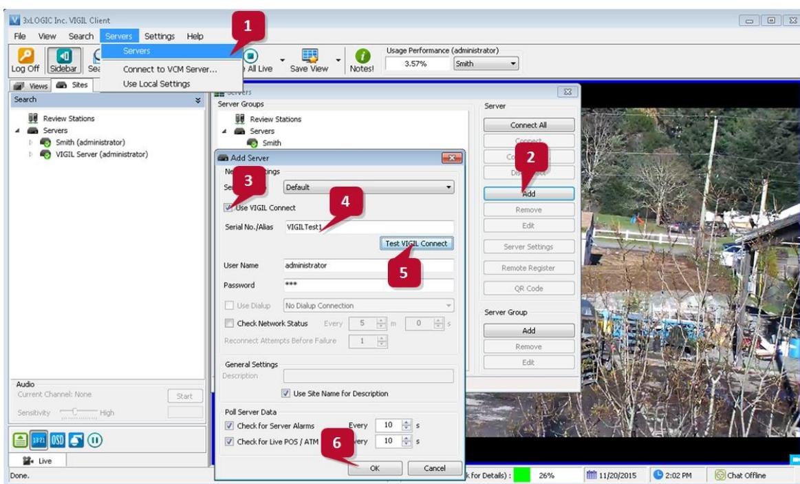
**Figure 4-4:** Adding V-Series Camera to VIGIL Client
